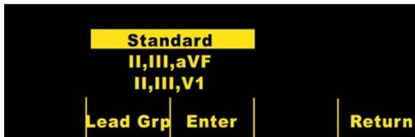
Press the **Lead Grp** softkey to scroll through and highlight the different Lead Group selections for three channel printing.
