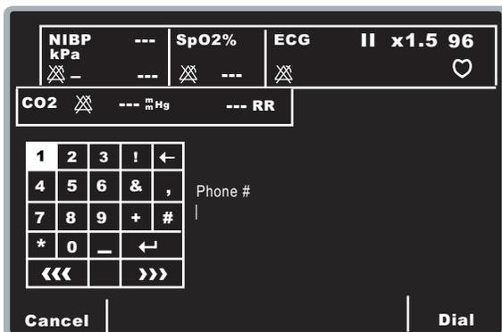
Use the scroll keys on top of the unit to select a number or character on the keypad, then press the **Commit** (⊙) key on top of the unit (see the next figure) to enter the digit in the Phone # field. Repeat for each additional digit (up to 20 characters).
