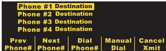
Press the **Prev Phone#** and **Next Phone#** softkeys to scroll the highlight up and down through the preconfigured phone/fax destinations.
