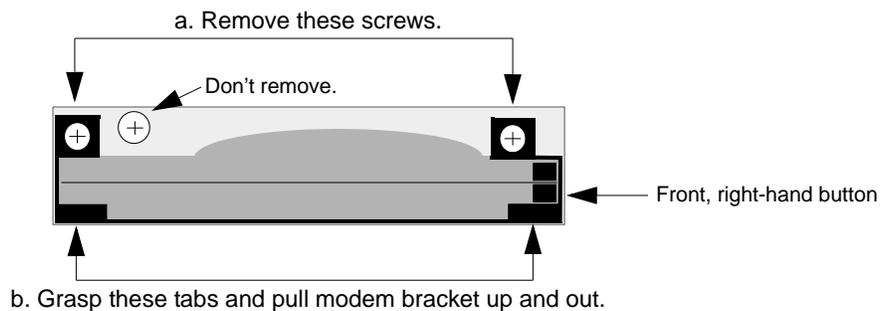
2. Press down on front right button to remove modem card.
