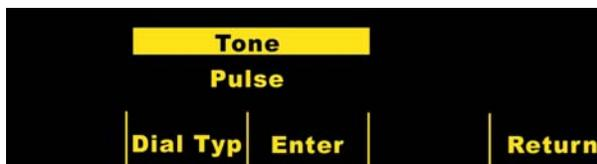
Press the **Dial Type** softkey to toggle between both types of dialing modes. Press the **Enter** softkey to save the highlighted dial mode and return to the 12 Lead Monitor menu. If you want to return to the 12 Lead
