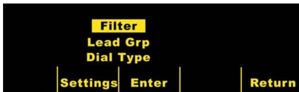
Once the settings screen is displayed, press the **Settings** softkey again to scroll through and highlight the different available selections. Press the **Enter** softkey to select the setting that is highlighted. You can return to the 12-lead Monitor screen by pressing the **Return** softkey.
