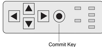
When you have entered the phone number, select the **Enter** (↵) key from the keypad and press the **Commit** (⊙) key on top of the unit to initiate dialing, or press the **Dial** softkey.
