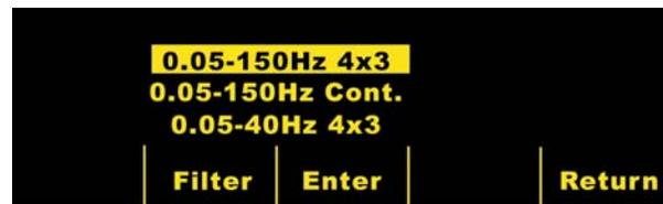
Select the filter you want to use by pressing the **Filter** softkey. The highlight area scrolls among the different filter choices. Press the **Enter** softkey to save the highlighted filter and return to the 12 Lead Monitor sub-menu.
