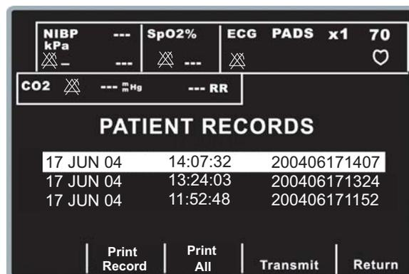
Use the scroll keys on top of the unit to navigate through the list of stored 12-lead records.
