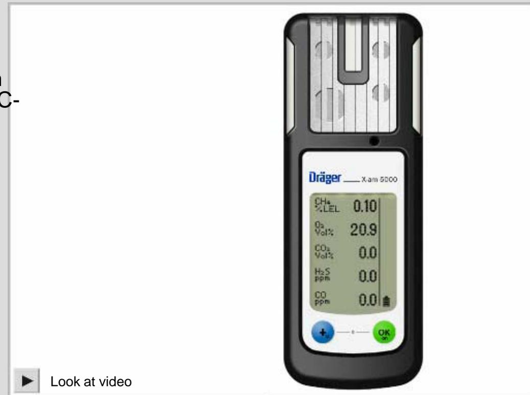
The fresh air calibration / zero point adjustment is not supported by the DrägerSensor Dual IR-CO2 and the DrägerSensor IR-CO2. A zero point calibration / adjustment of these sensors can be conducted using the Dräger CC-Vision PC software. To do so, a suitable zero gas that is free of carbon dioxide (e.g. N2) should be used.
