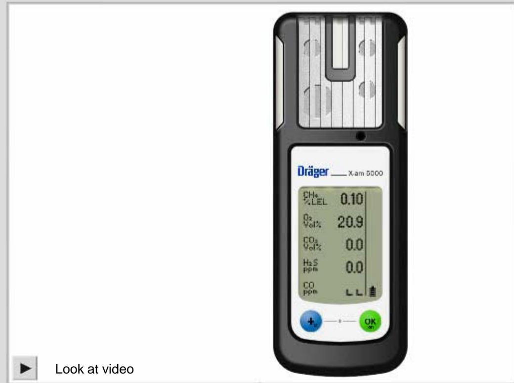
The measured concentration has drifted into the negative range. This can e.g. happen, when the fresh air calibration was done in an area where a concentration of gas was present. Please fresh air calibrate the instrument in a clean environmental.
