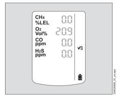
After the preset bump test concentration is reached or a gas alarm is triggered (with the "Quick bump test"):
