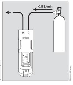
Upon application of the Dräger mixed gas (order no. 68 11 130) the displays should be within this range.
