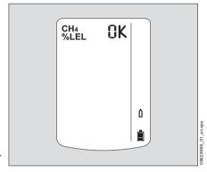
Close the test gas cylinder valve and remove the device from the calibration cradle.
