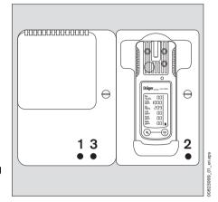
A short circuit of the charging contacts in the charging modules, e.g., by metallic objects that have fallen in, does not result in damage to the charging station. It should, however, be avoided due to possible heating hazards and incorrect displays on the charging module.
