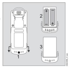
After replacing the power pack T4, it is recommended that a complete charging is carried out.
