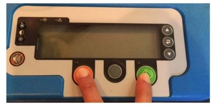
2. USE THE DOWN ARROW TO SCROLL DOWN TO "ROTATE SHAFT TO HOME" AND THEN HIT THE ENTER KEY ABOVE THE DOWN ARROW:
