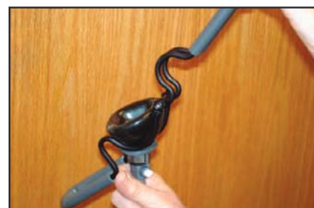
Count to 10, push white purge valve & black bulb should re-inflate.
