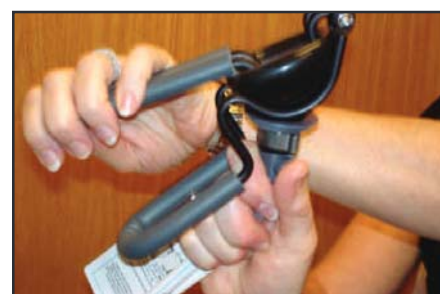
Press the black ball while holding down the white purge valve.
